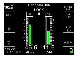
• Press the ID soft key to verify the satellite. "ID VERIFIED" means you are pointed correctly.
